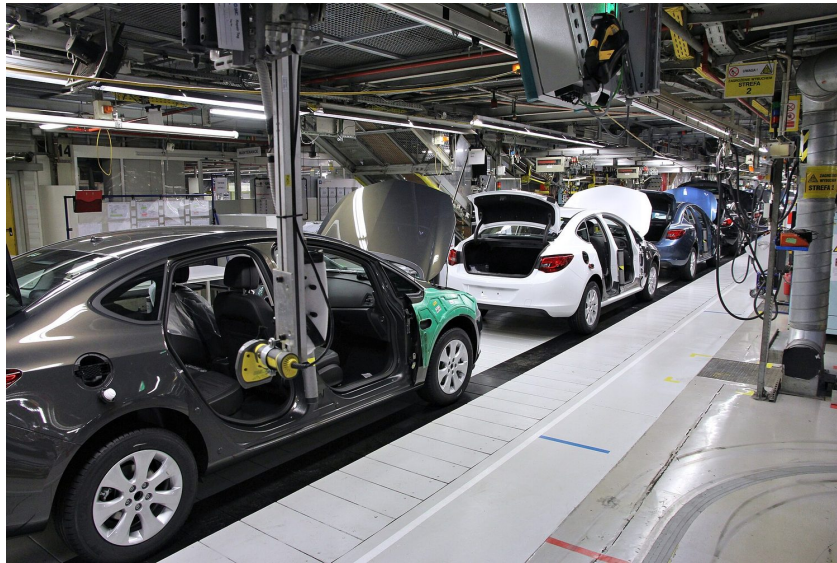
A car assembly line: flow production of identical units, one stage after another
