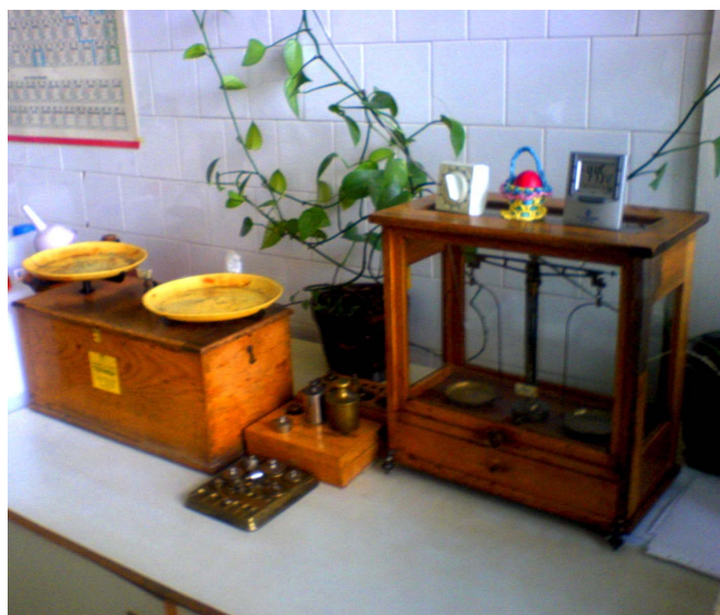
A laboratory balance measures mass —the basis of mole calculations.
