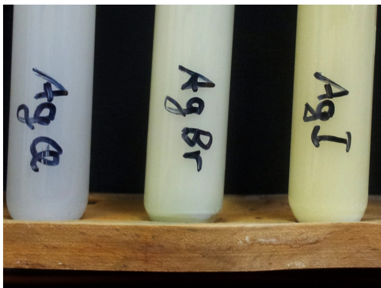
The silver halide test: AgCl is white, AgBr cream and AgI yellow
