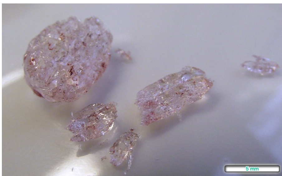
Phenol is a low-melting solid; it slowly turns pink as it oxidises in air
