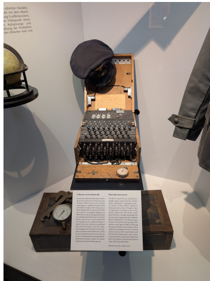
The Enigma machine encrypted messages in the Second World War —an early, mechanical cipher device
