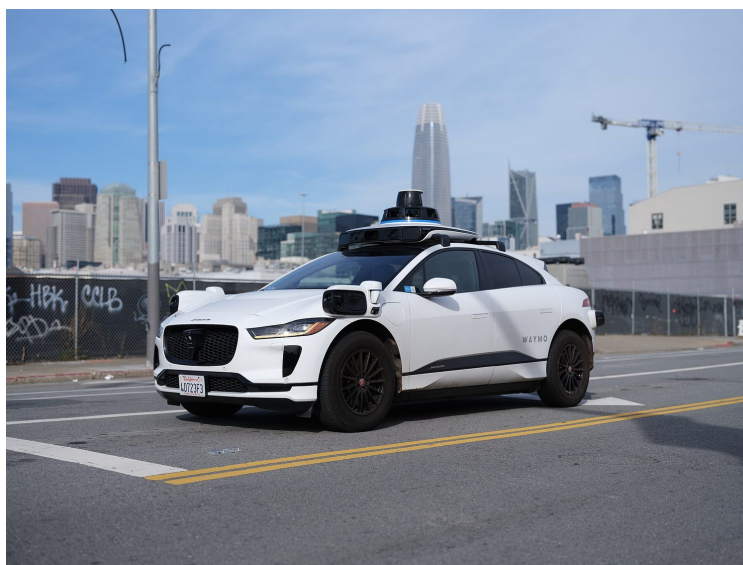
A self-driving car uses cameras and lidar sensors to see the road around it
