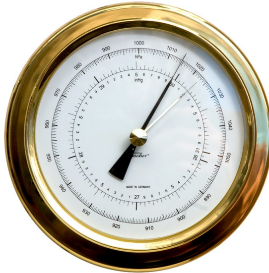
A precision aneroid barometer measures atmospheric pressure
