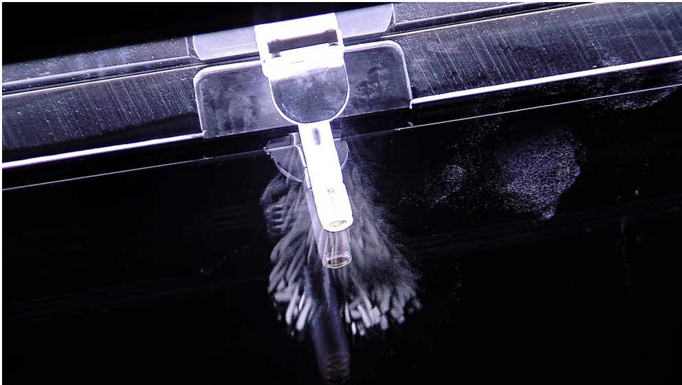
Alpha-particle tracks in a cloud chamber, fanning out from an americium-241 source
