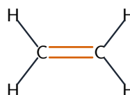
ethene C_2H_4 unsaturated: C=C double bond
